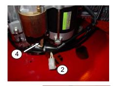
36" belt drive blade activation safety switch location top view.
