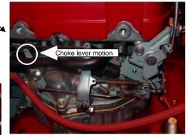
Above: 36" Honda Mower Throttle and Choke Connection
