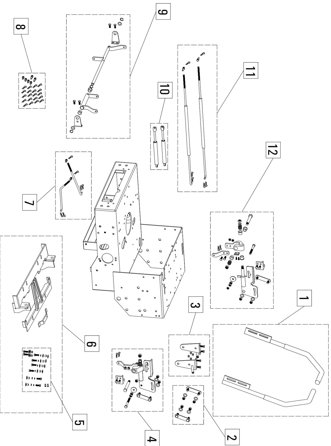
**54ZS" Chassis Diagram -Hydrostatic Drive Controls Key**
