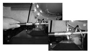
4. Press the cable toward the chute rotator screw. The end of the cable should touch the end of the chute rotator.
