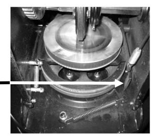
IMPORTANT! The snow blower belts are adjusted to ensure the augers stop turning within 5 seconds of releasing the augers/impeller control lever. If you are making any belt adjustments whatsoever, for your safety and the safety of others around you, you must ensure the belts are re-adjusted to achieve this design specification.
