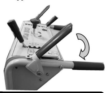
IMPORTANT! The snow blower belts are adjusted to ensure the augers stop turning within five (5) seconds of releasing the impeller control lever. If you are making any belt adjustments whatsoever, for your safety and the safety of others around you, you must ensure the belts are re-adjusted to achieve this design specification.
