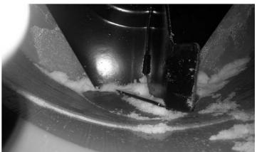
If the impeller is frozen up when the impeller / collector handle is engaged, the belts will bog down the engine and the belts will begin to burn on the engine pulley since they cannot move, or a shear pin could fail.
