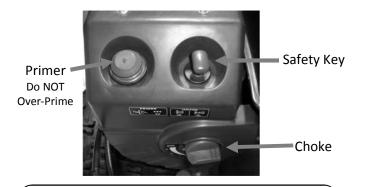
Do NOT over-prime the engine. Pressing the primer bulb more than 3x could result in flooding the carburetor making the engine hard to start or cause fuel to leak from the carburetor inlet.
